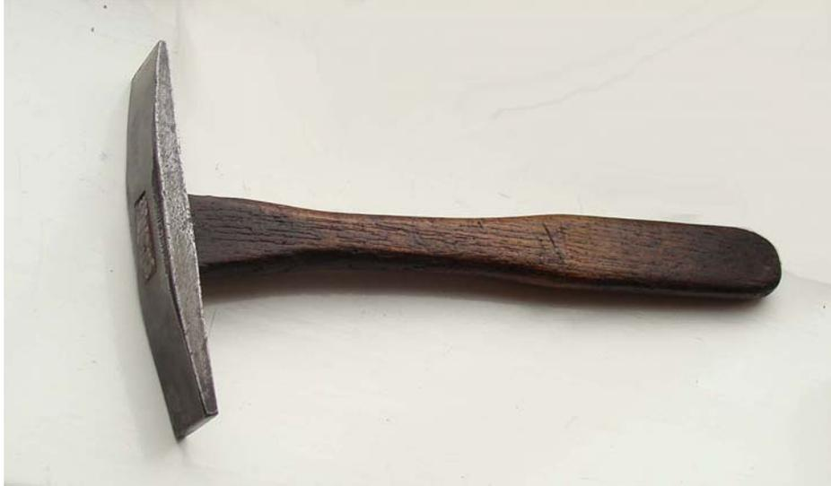
hammer and then turning the blade over and hitting the alternate teeth. Years of practice gave enough skill to set the teeth rapidly at a low cost.
